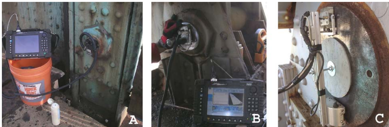
Figure 8: (A) small pin scanner (B) medium pin scanner (C) large pin scanner
